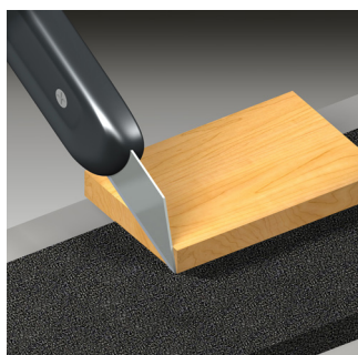
Figure 3: To accommodate setting blocks, notch out tape
